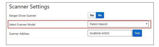
**5.** Type **localhost:44343** into the **Scanner Address** textbox if using Internet Explorer<sup>®</sup>. Click **Test**.
